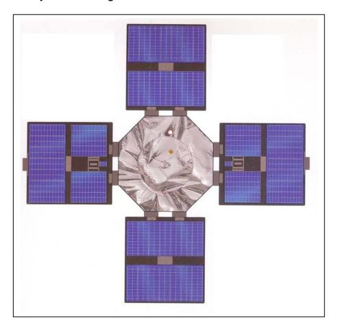
NASA's twin Van Allen Probes spacecraft will be launched in 2012. The figure above shows the octagonal spacecraft body and the location of the surrounding four solar panel 'wings' that provide power to the spacecraft instruments. The small blue rectangles within each of the four solar panels show the location of the solar cells used to power the satellite. As the spacecraft orbits Earth, the four solar panels continuously face the sun to provide constant power.
