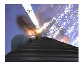
The Juno spacecraft was launched on August 5, 2011 on a 5 year journey to Jupiter. This image was taken 120 seconds after launch and shows one of the solid rocket boosters being jettisoned. The camera is on the Atlas booster and looks down on the engines and the distant arc of a cloudy Earth. Scenes from the launch can be found on YouTube. and show a dazzling launch from multiple viewing locations on Earth and in space.
