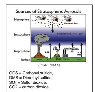
SAGE-III is designed to measure the concentration of aerosols in the stratosphere, but where do these particles come from?
