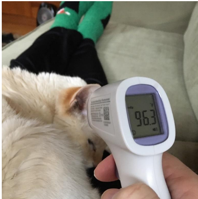
Figure 57 – Measuring the temperature of a surface with a non-contact IR thermometer. This healthy cat has a temperature of 96.3° F and was not at all bothered by the measurement! (Credit: Sten Odenwald).
