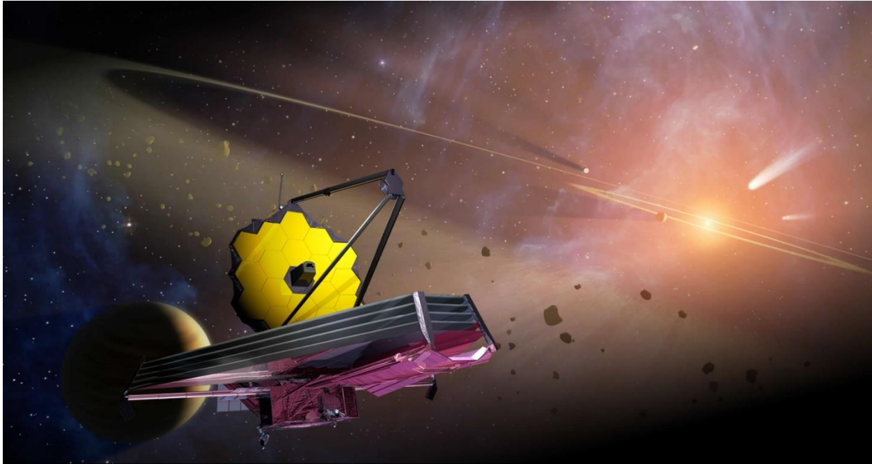
Figure 2 - Artistic rendering of the James Webb Space Telescope, showing the primary mirror and multi-layered sun shield. (Credit: NASA)
