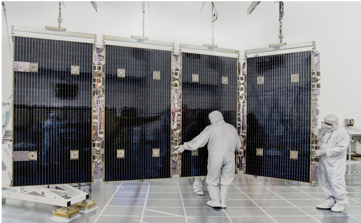
Figure 41 – Technologists holding the solar array of the James Webb Space Telescope after a test of the array earlier in 2020. The fifth panel of the solar array is folded behind the fourth in this image. (Credit: NASA/Chris Gunn)
