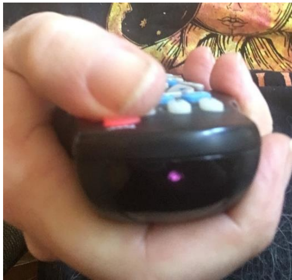
Figure 56 – A common TV remote unit emits an infrared beam. You can't see it with your eye but a photo taken with the selfie camera has enough infrared sensitivity to discern its pulse of light. (Credit: Sten Odenwald)
