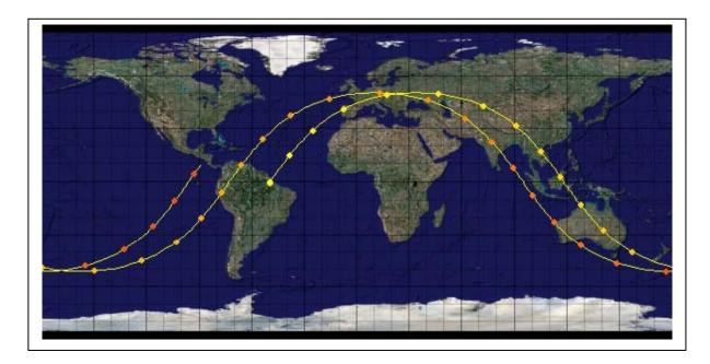
As the ISS orbits Earth every 90 minutes, Earth rotates 'underneath' the orbit of the ISS once every 24 hours. This means that each ISS orbit advances in longitude by a fixed amount in longitude. The figure above shows the ground track of the ISS for two orbits. Each square is 10 degrees on a side, with the Equator running horizontally across the middle of the diagram. The squares are shown at intervals of 5 minutes.
